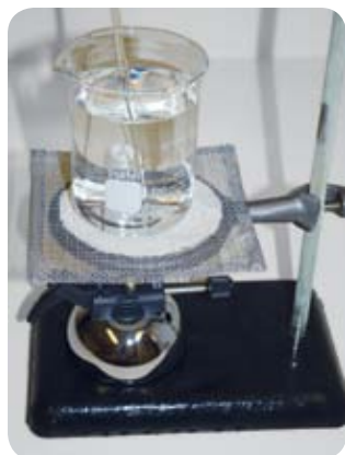
FIGURE 5-16: Using a stirring rod to avoid superheating
