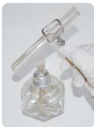
FIGURE 5-17: Heating a test tube properly
