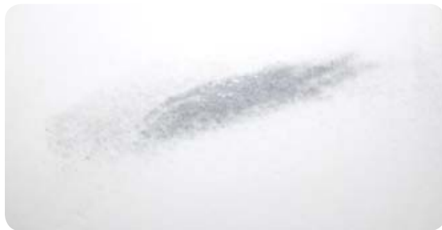
FIGURE 22-6: A positive Marsh Test for arsenic
