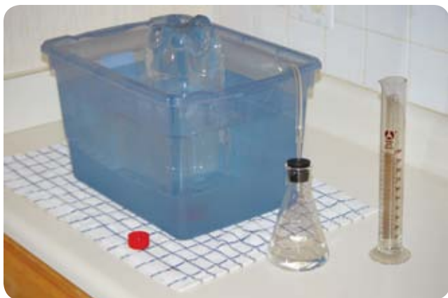
FIGURE 14-5: My apparatus for gas generation and collection
