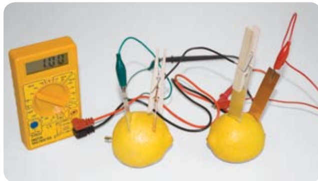
FIGURE 16-5: A two-cell series lemon-powered battery
