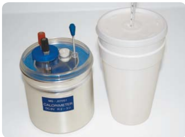
FIGURE 15-1: Store-bought (left) and homemade calorimeters
