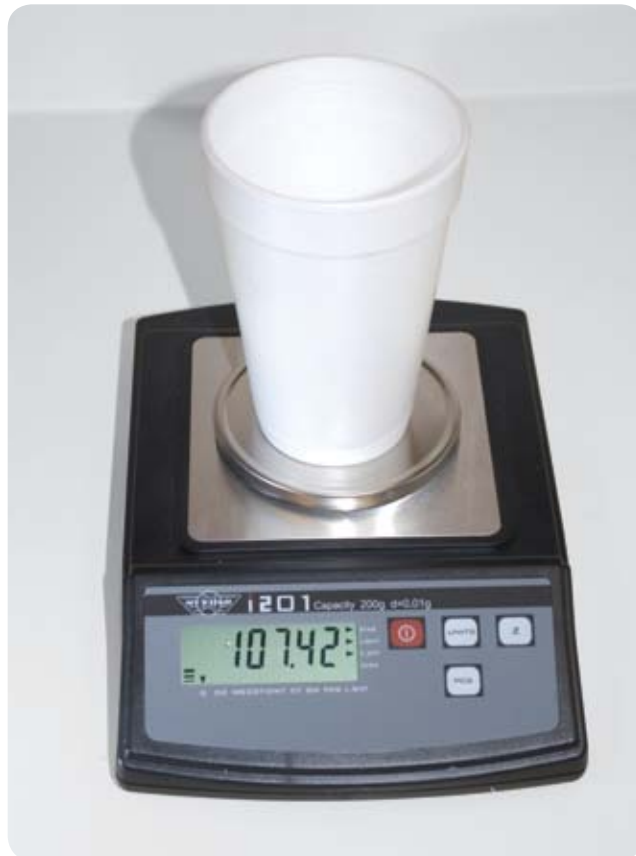
FIGURE 12-1: Observing the mass change as the Alka-Seltzer tablet reacts and carbon dioxide is evolved
