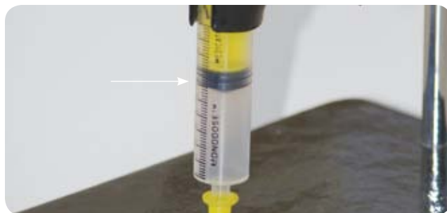
FIGURE 14-2: Measure the gas volume at the lowest bearing surface of the plunger
