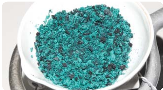
FIGURE 10-1: Mixed copper carbonate and charcoal before smelting
