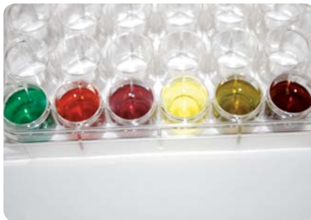
FIGURE 22-2: A spot plate showing positive and negative results for various substances
