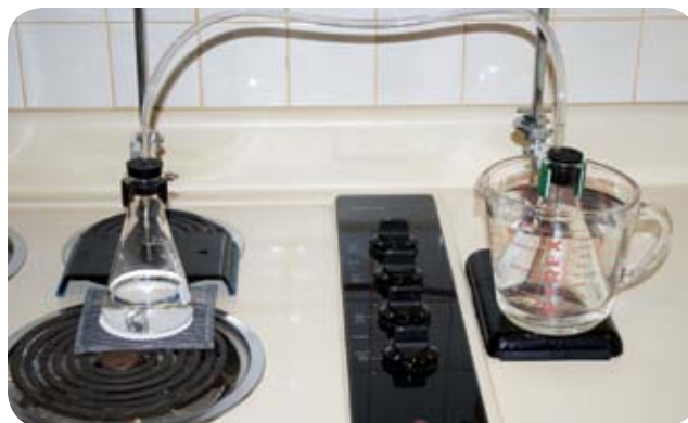
FIGURE 6-2: My distillation apparatus
