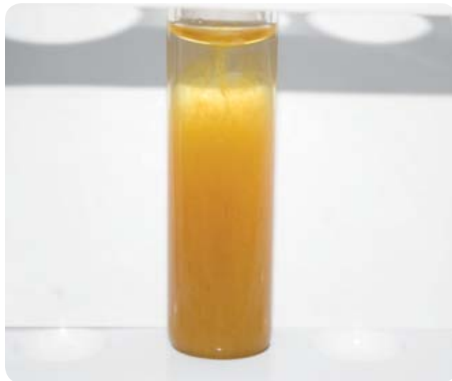
FIGURE 19-3: A yellowish precipitate upon addition of ammonium molybdate confirms the presence of phosphate ions
