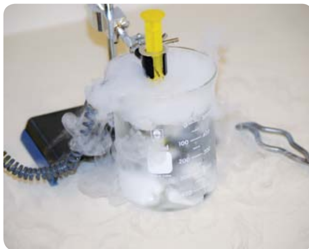
FIGURE 14-3: Measuring gas volume in a bath of alcohol and dry ice
