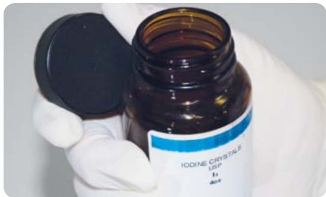
FIGURE 5-1: Hold the cap, rather than placing it on the bench
