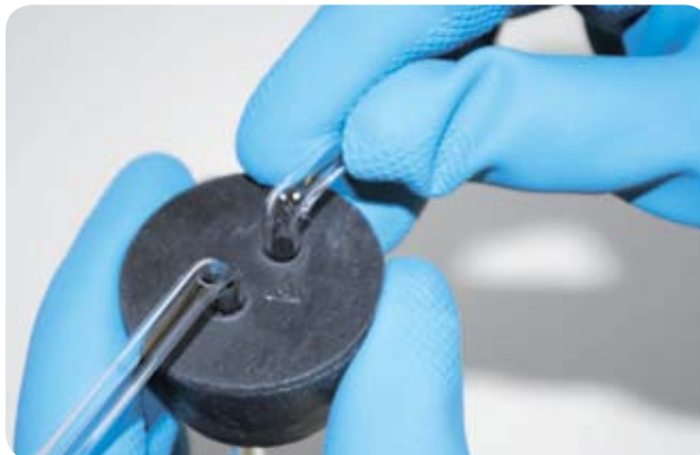
FIGURE 5-25: Lubricate the glass tubing with glycerol or oil and then rotate it as you slide it into the stopper
