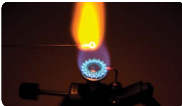
FIGURE 19-1: A positive flame test for sodium
