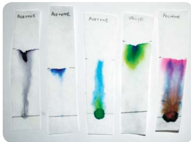
FIGURE 6-6: These chromatograms show the separation of the ink and food coloring components with polar (water) and nonpolar (acetone) solvents
