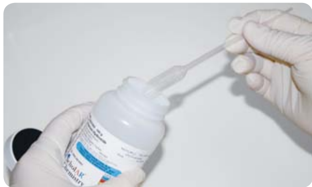
FIGURE 5-3: Use a modified Beral pipette as a scoop
