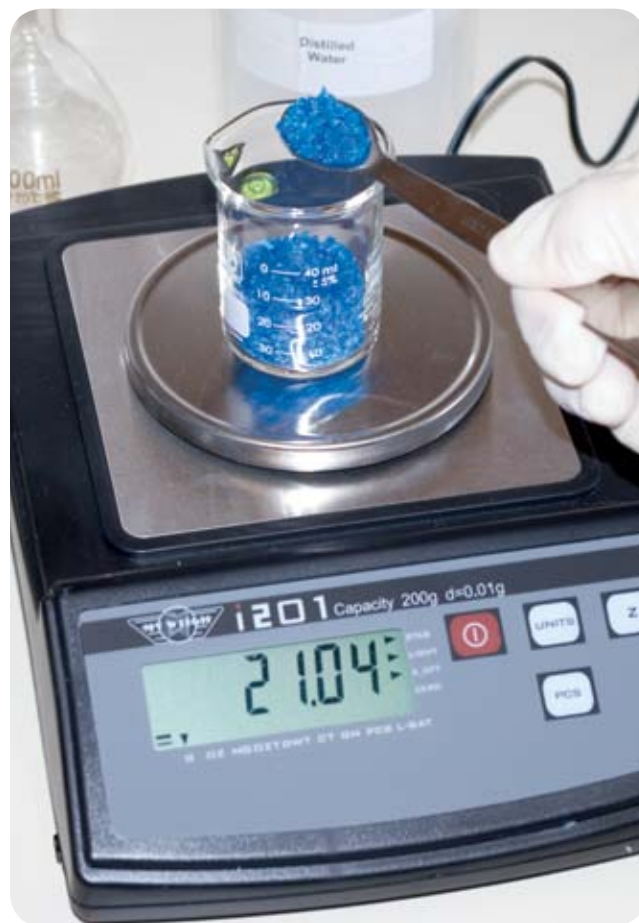
FIGURE 7-1: Weighing the sample of copper sulfate
