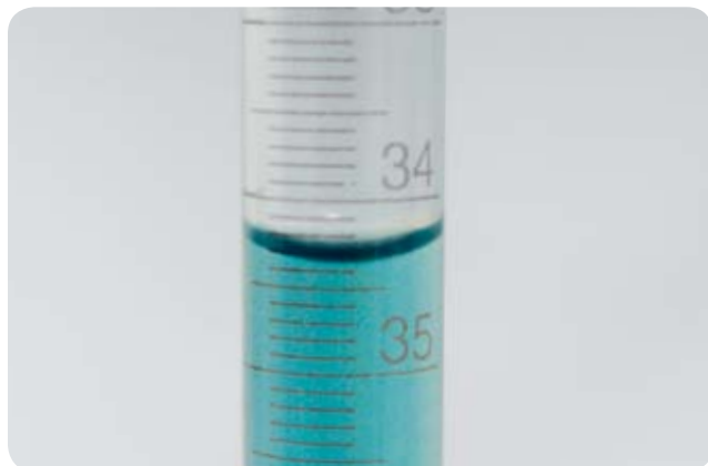
FIGURE 5-10: Reading the meniscus on a burette
