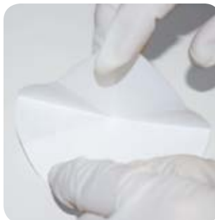
FIGURE 5-13: Making a filter paper cone
