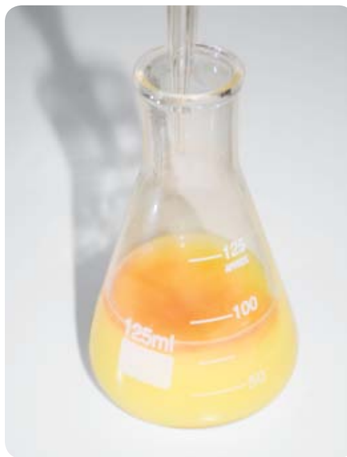
FIGURE 20-2: The first appearance of silver chromate tints the solution orange
