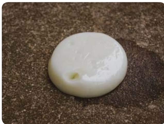
FIGURE 18-5: Although it is technically a liquid, the gelled sol maintains its form as though it were a solid
