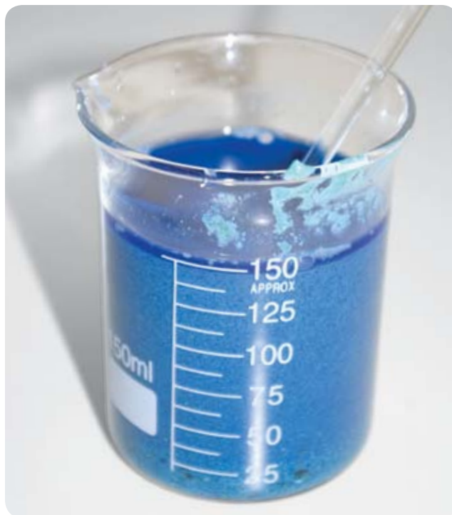
FIGURE 9-6: Schweizer's Reagent, formed by reacting copper(II) hydroxide with aqueous ammonia
