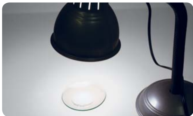
FIGURE 5-19: Using a lamp to dry a sample
