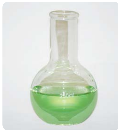
FIGURE 3-6: A 250 mL flat-bottom Florence flask
