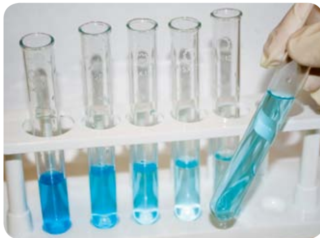
FIGURE 7-5: Comparing the solution of unknown concentration against samples of known concentration
