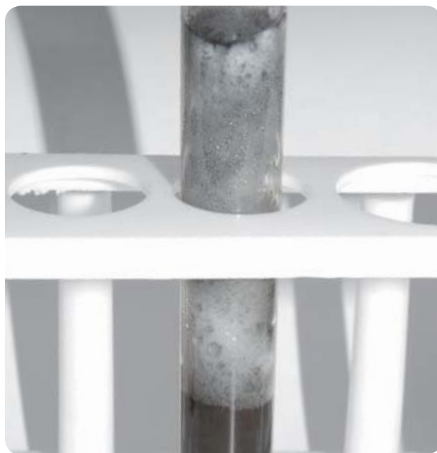
FIGURE 9-3: Aluminum metal reacting with hydrochloric acid
