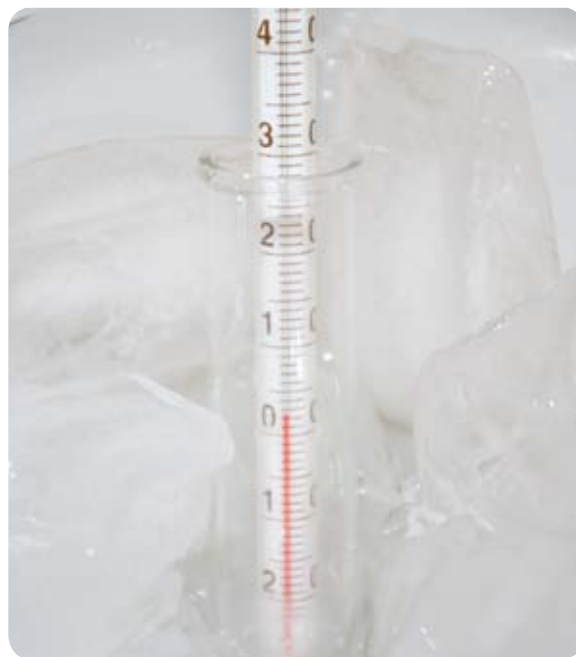
FIGURE 8-2: Determining the freezing point of a solution
