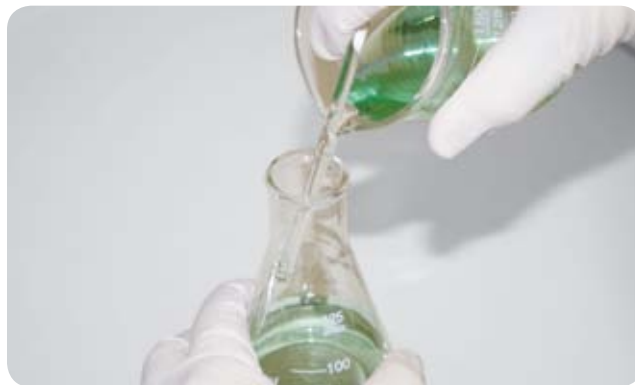
FIGURE 5-4: Using a stirring rod to transfer a liquid
