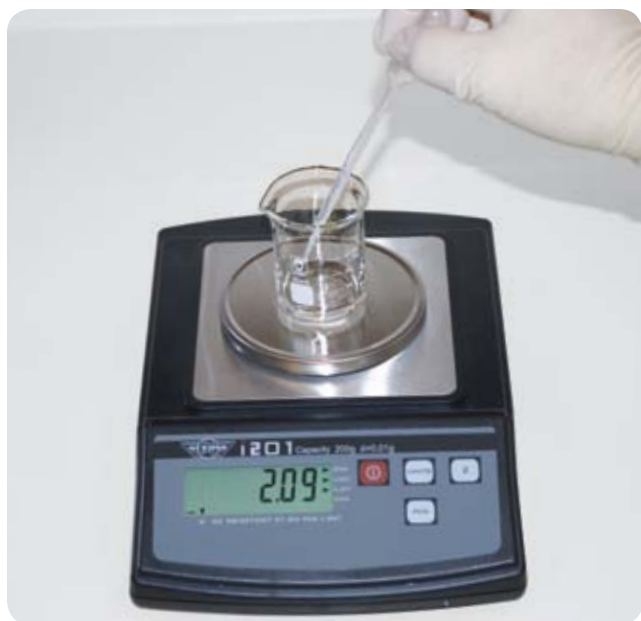
FIGURE 5-9: Calibrating a disposable pipette
