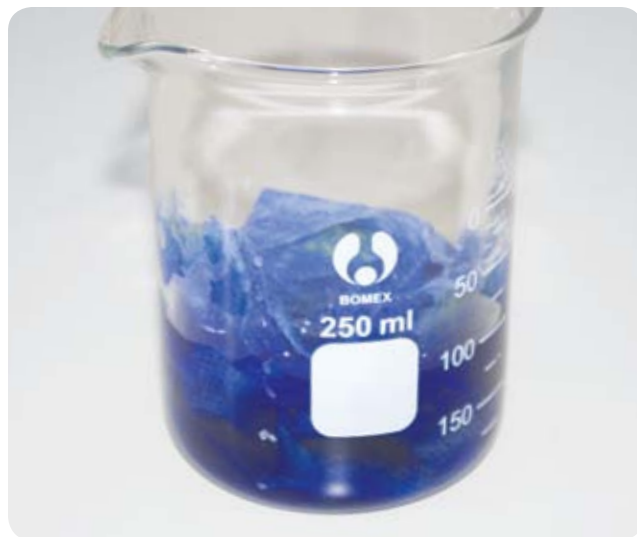
FIGURE 21-3: Dissolving cellulose (paper) in a solution of Schweizer's Reagent
