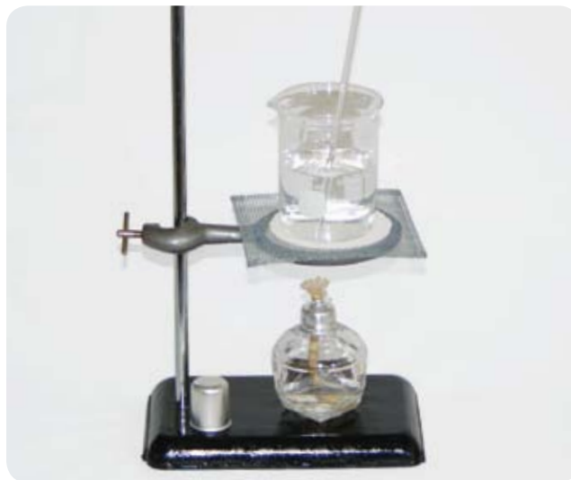
FIGURE 3-4: Use a stirring rod to prevent boiling over
