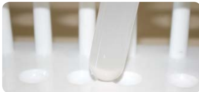
FIGURE 19-2: A white precipitate upon addition of barium nitrate confirms the presence of sulfate ions
