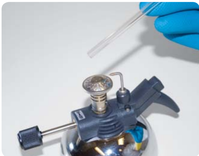
FIGURE 5-22: Rotate the end of the glass tubing in the flame to smooth the edges
