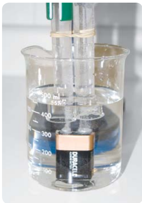
FIGURE 16-1: A homemade version of a commercial Brownlee electrolysis setup
