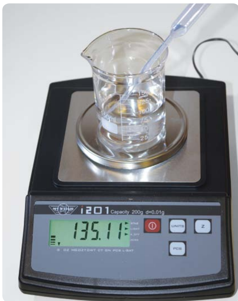
FIGURE 5-12: Determining the combined mass of beaker, titrant, and Beral pipette
