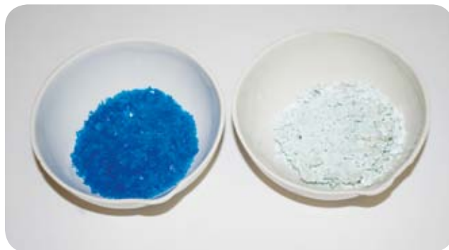
FIGURE 6-7: Copper sulfate samples before (left) and after heating (right) to remove water of crystallization
