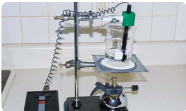
FIGURE 8-1: Determining the boiling point of a solution
