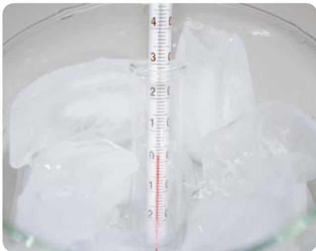
FIGURE 21-2: Determining the freezing point of the semi-pure methyl salicylate
