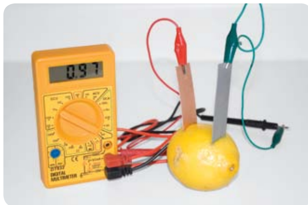
FIGURE 16-2: Measuring the voltage produced by an electrochemical cell with copper and zinc electrodes (note that the actual voltage is lower than the theoretical 1.10V)
