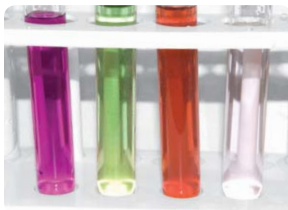
FIGURE 10-2: Oxidation states of manganese
