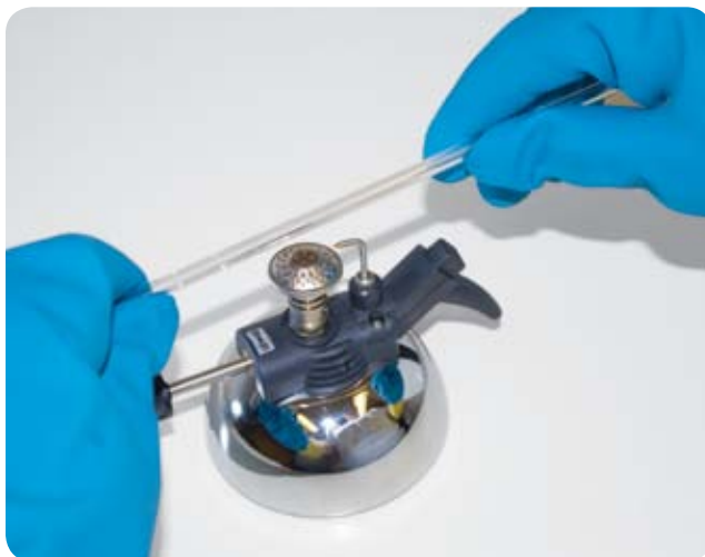
FIGURE 5-23: Heat the section of the glass tubing to be bent by rotating it in the flame
